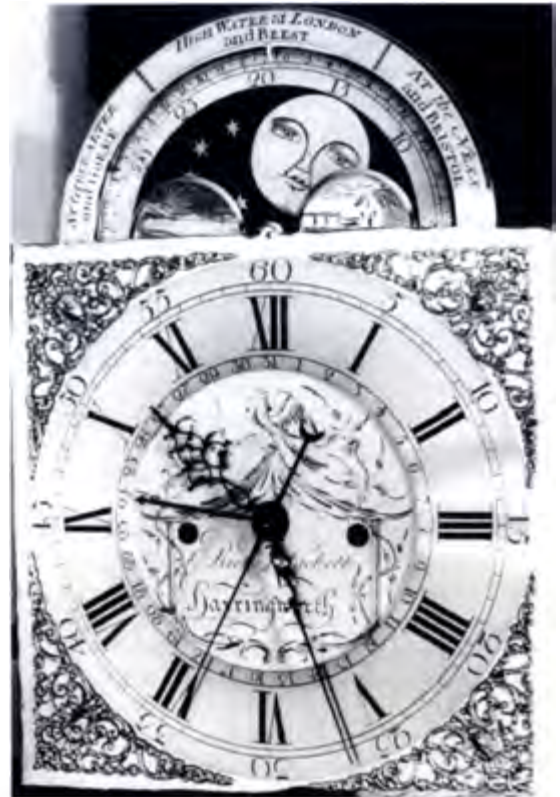
The dial of Richard Hackett's eight-day longcase clock which has a moon with tidal readings for six different ports. Note the centre seconds and date hands (Loomes 1985, 180)
