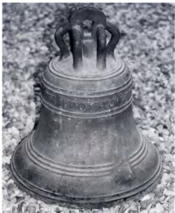
The former clock bell at Morcott. Note the indentation as a result of being struck by the clock hammer
