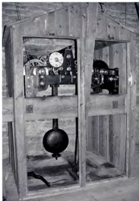
The present movement at Ashwell Church by Thwaites and Reed of London
