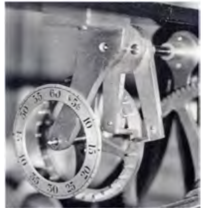
The pinwheel escapement and seconds dial
