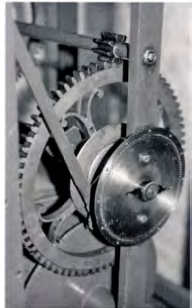
The setting dial and first wheel of the going train of the Normanton Park Hotel clock. Note the interesting wheel crossing
