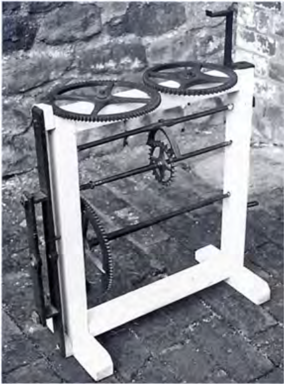
The parts removed during the restoration and conversion to verge and foliot escapement
