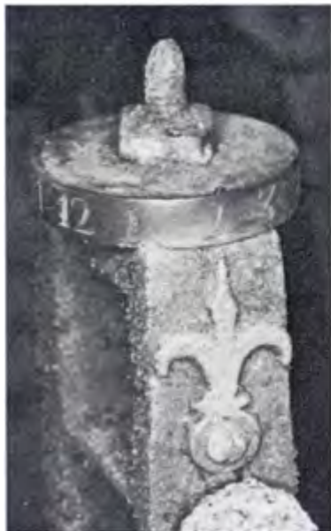
The pendulum suspension bracket and rating nut on the Burley clock (Chris McKay)
