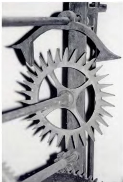
The anchor escapement of the John Watts clock at Clipsham
