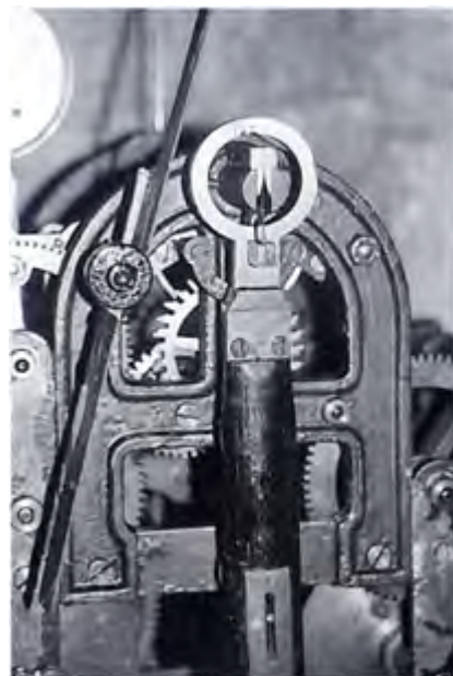
The pendulum suspension and the going train remontoir fly on the Phil Horz clock at Edith Weston
