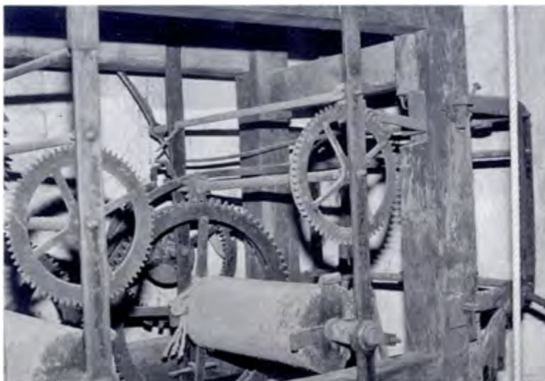
A close-up view of the strike train of the former Empingham church clock, now in Stamford Museum. It is signed I W 1686 indicating that it was made in 1686 by John Watts of Stamford (Lincolnshire County Council: Stamford Museum 31/2/26)
