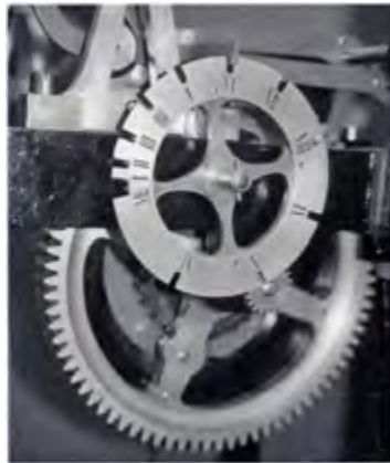
The numbered countwheel
