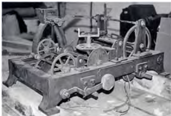
The former two-train clock movement at Hambleton Hall stables by John Smith & Sons of Derby. The movement was removed from a room below the clock turret when the stables were converted. A synchronous electric movement now drives the hands
