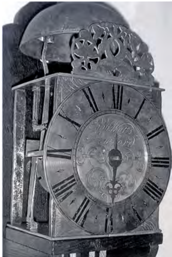
A rare transitional lantern clock of circa 1730 by Robert Watts of Stamford (Philip Snowden). Like his thirty-hour longcase clocks, it has an anchor escapement, long pendulum and posted frame movement. However, it was made to look like a lantern clock by the use of a lantern type dial and a single front fret. It is designed to sit on a wooden wall bracket. The use of iron for the bell standard and the vertical frame bars, and the deletion of expensive brass finials, side frets, side doors and feet, made this a very much cheaper clock. This clock is described by Brian Loomes in Clocks (2002, 16-19)
