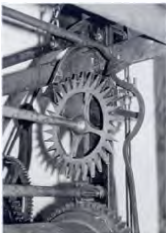
(left) Ryhall Church. The anchor escapement of William Bird's clock
