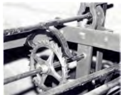
The anchor escapement of Caldecott church clock
