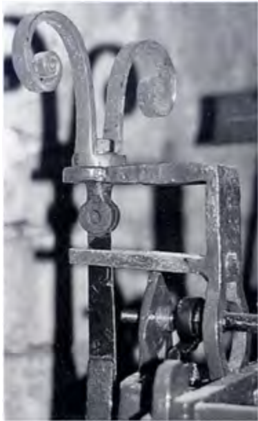
The rating butterfly at the top of the pendulum of Caldecott church clock is similar to those seen on Eayre clocks
