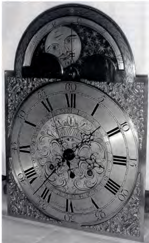
The dial of a Richard Hackett eight-day longcase clock with centre seconds and date hands (Philip Snowden)
