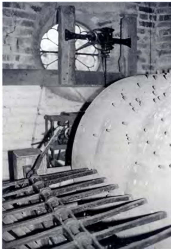
(above) The six-tune chime barrel by Edward Arnold at Stapleford Church, Leicestershire. It has twelve chime levers which are connected to bell hammers in the belfry by wires and bellcranks and each bell has two bell hammers. The names of the tunes are recorded on a brass plaque on the frame and the barrel is still used today for weddings and concerts
