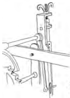
A top pendulum adjuster on a turret clock of circa 1760 (Chris McKay)
