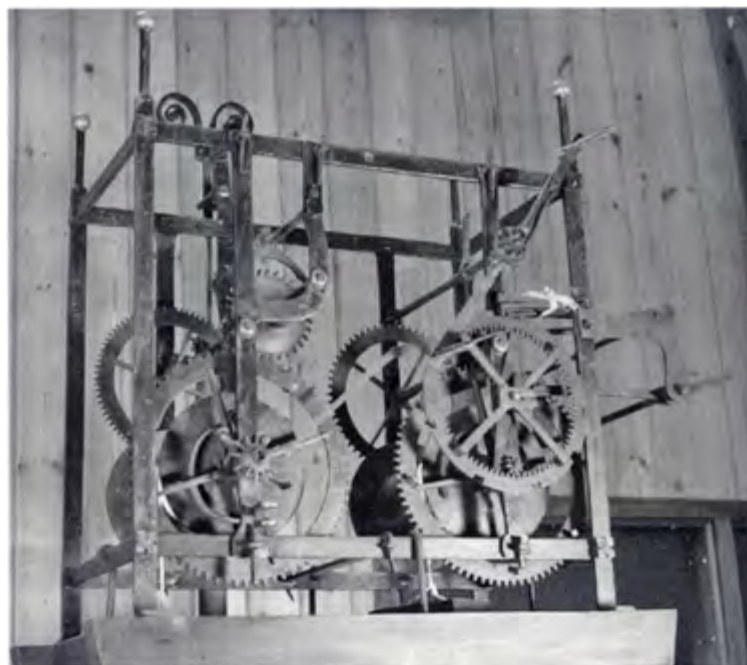
The birdcage clock movement by Thomas Eayre II from Loddington Hall stables. It is now on display in Rutland County Museum (1969.428)
