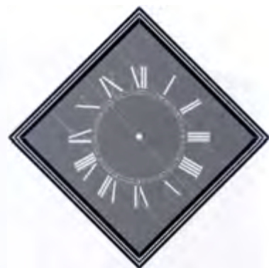
A typical John Watts dial consisted of four planks with four lengths of edge moulding. These would be assembled and decorated in the workshop and, like the clock frames, could be dismantled for easy transport
