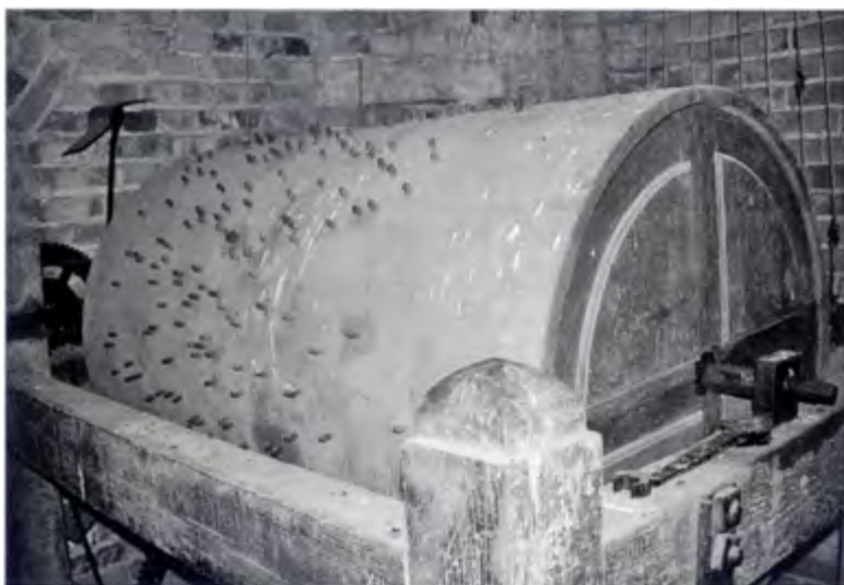
(above) The six-tune chime barrel by Edward Arnold at Stapleford Church, Leicestershire. It has twelve chime levers which are connected to bell hammers in the belfry by wires and bellcranks and each bell has two bell hammers. The names of the tunes are recorded on a brass plaque on the frame and the barrel is still used today for weddings and concerts
