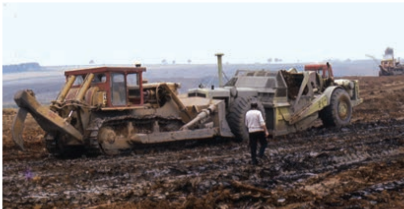
Left: A heavily loaded Terex motor scraper gets a push from a bulldozer (Brian and Elizabeth Nicholls Photography)
