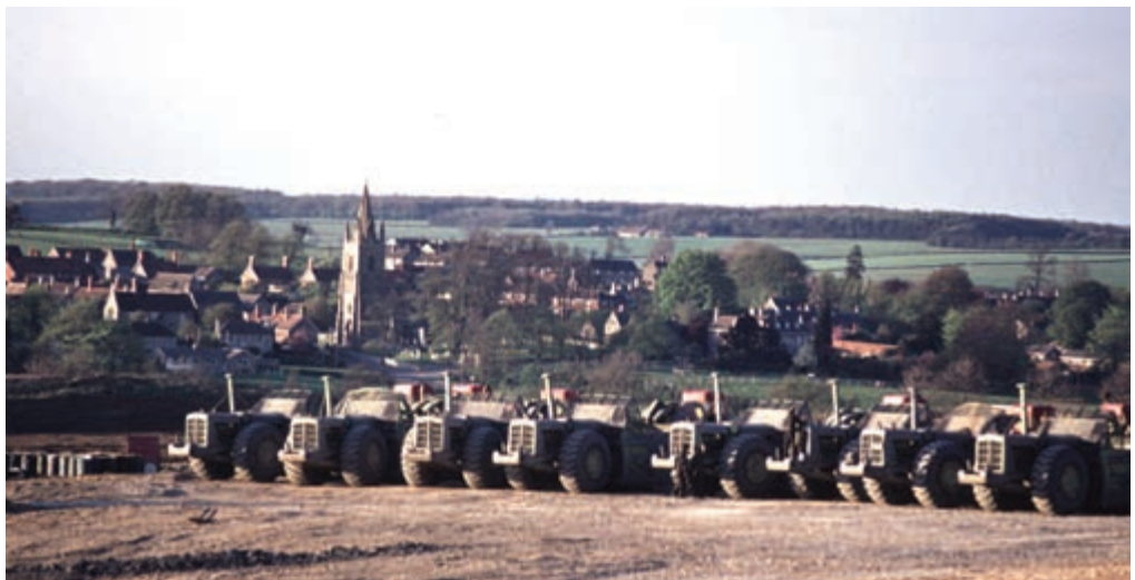
Right: Seven of the 12 twin-engined Terex motor scrapers ready for work. View looking from the dam towards Empingham (Brian and Elizabeth Nicholls Photography)
