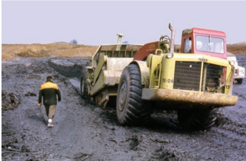
One of the Terex motor scrapers emerging from a borrow pit near the dam site (Brian and Elizabeth Nicholls Photography)
