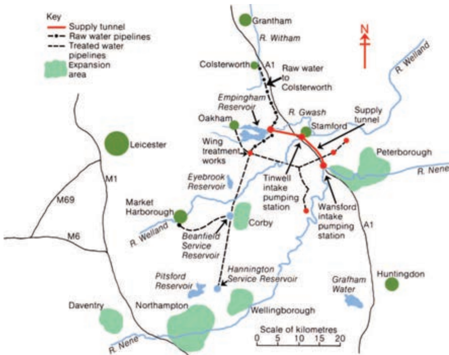
The Empingham Pumped Storage Project (after the Institution of Civil Engineers)
